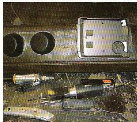
4. The SAVV 5.6-inch TV pod and gauge pods are held in place using CA glue.
