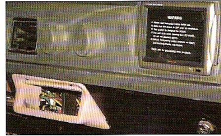
16. The dash is now back in the car for a test fit. It has been sanded smooth and is ready for texture and paint.
