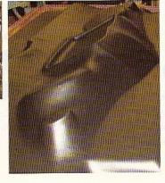
9. I heated up a sheet of .140-inch ABS plastic in an oven and draped it over the mold. I applied vacuum and sucked the hot plastic around over the mold, making sure not to get plastic underneath so it can be removed easily once the plastic has cooled a little. The result is a plastic housing that is light, easy to paint or cover and very cool!
